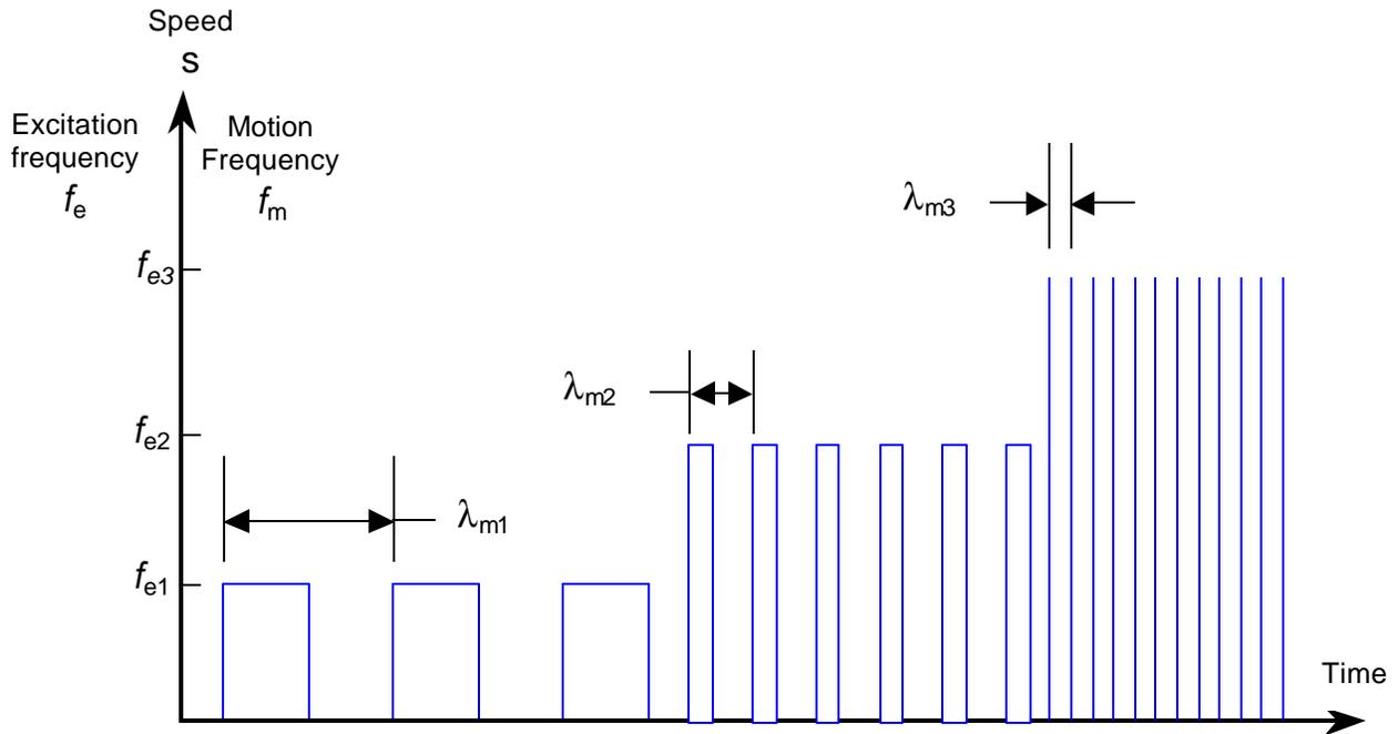
FIG. 2 Excitation frequency  $f_e$ , represents the frequency of nerve impulses,  $s$  the speed of the aluminum structure,  $f_m$  the frequency of motion of the aluminum model. Note how the speed of the model  $s$  and the motion frequency  $f_m$  increase as the input excitation frequency increases.
