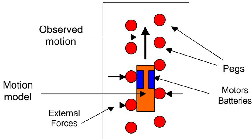
Fig. 2 Harmonically excited motion model moves normally to externally applied forces
