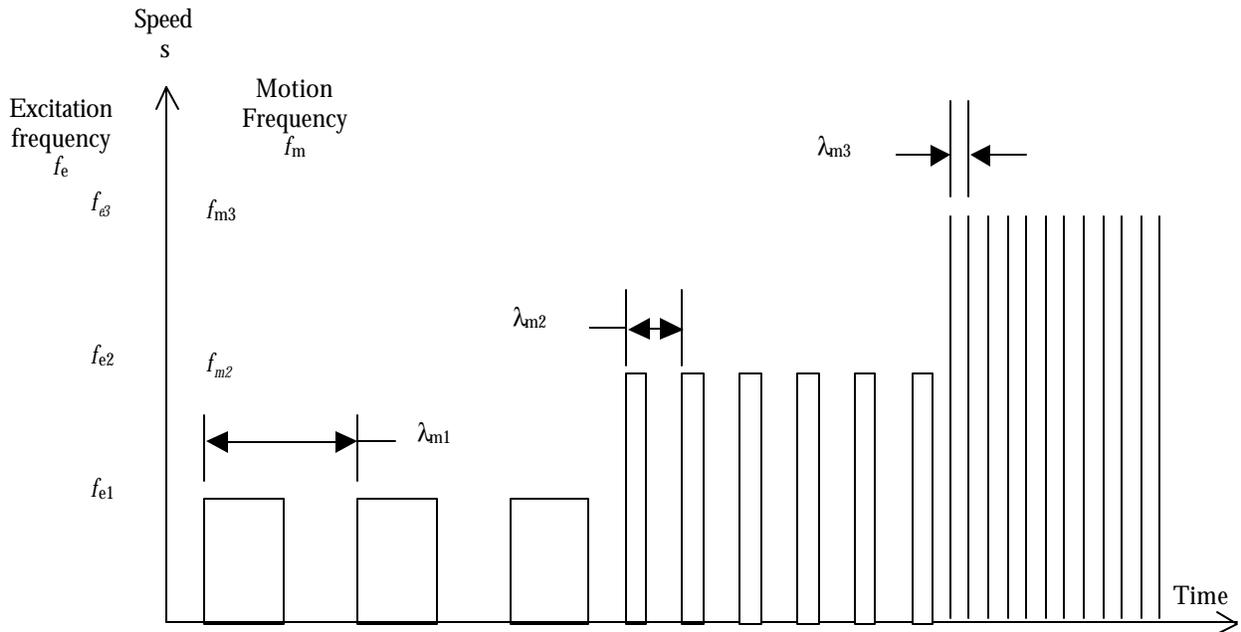
FIG. 2 Self-motion explains quantum effects. Notice the two distinct frequencies and the two distinct wavelengths; (1) the excitation frequency  $f_e$  which causes the motion and (2) the motion frequency  $f_m$  which results from the discrete motion.
